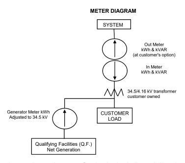
All meters are detented so only power flowing in the indicated direction is measured. Generator Meter readings are multiplied by 1.003 to bring them to the same voltage as the In Meter.
